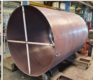
Figure 7 - 3D view of an IJS (left), coupling side of the steel cylinder (centre) and detail of the metal cross (right)
